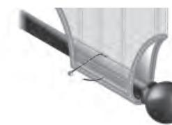
3) Make sure the rod is seated in the bottom of the loop. Once installed, the cable ties cannot be adjusted. Insert the ends of the cable tie together and tighten. Clip off the tail.
