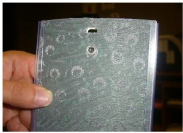
If the hole is stretched or is too large for the clear insert button, the louvers must be reordered.
