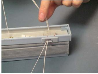
6. Remove cord from blind by pulling knot in bottomrail. Do not remove plastic washers. Match new cord to existing cord length in the shade. If unable to match, cut cord lengths using
