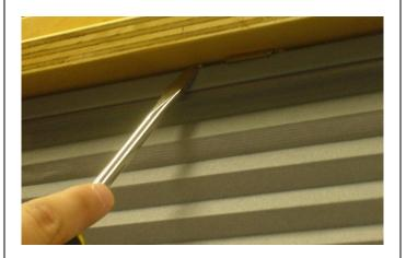
2. Unscrew the top joiner ball. Set aside danskord (thick rope cord). Untie joiner ball knot. Remove joiner ball and washer.
