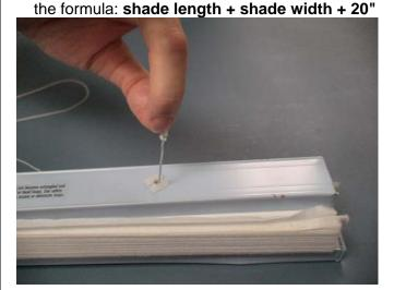
5. Use a pair of pliers to remove the cord lock. When removing, both sides of the cord lock should be pushed at the same time or push wing and move one side at a time.
