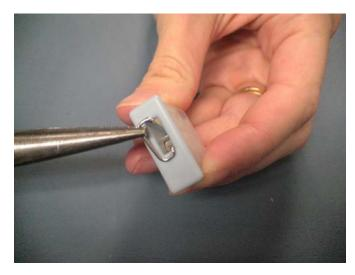
**10.** Feed the cord through the cord lock, making sure the cord is between the silver rivet and the roller in the cord lock.
