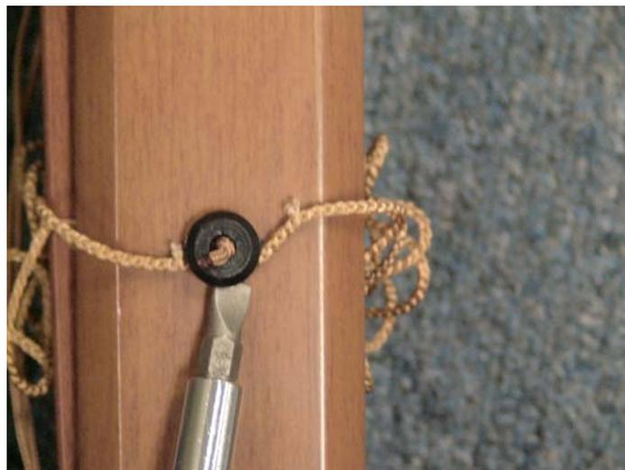
4. Locate slat just above the bottomrail to measure or locate the slat to be replaced. Reach between the ladders and pull lift cord out of the bottomrail and through the route holes just until cording is out of this slat. Continue for all lift cords on the blind.
