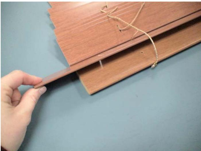
6. Using a metal tape measure, measure from the left end of the slat to the middle of the first route hole. Record this measurement to the nearest 1/16”.
