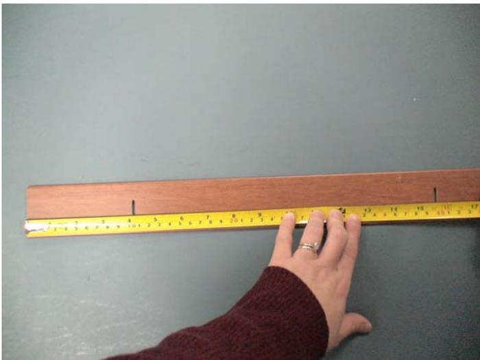
8. Continue in the same manner with the remaining route holes. Record all the remaining measurements. Record the overall width of the slat to the nearest 1/16”.
