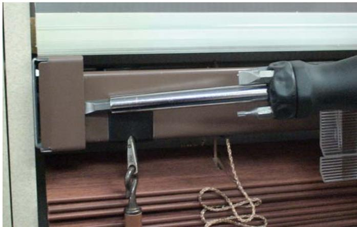
3. Use a flathead screwdriver to remove the bottomrail retainers. If there are cloth tapes, you will also need to remove the upholstery tacks. **DO NOT DISCARD TACKS.** Untie lift cord knots.
