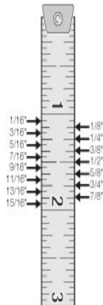
7. With the tape measure still on the left side of the slat, measure the middle of the second route hole from the left side of the slat. Record this measurement.
