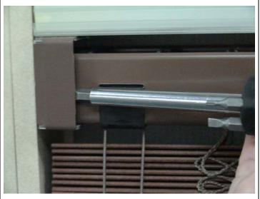
3. Check to make sure tilt rod is completely into the tilter mechanism. Tilt rod will be inserted so you can see it on both sides of the tilter mechanism.
